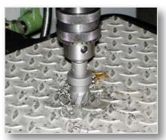
Drilling structured sheet metals
