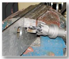
Free-hand drilling up to Ø 30 mm
