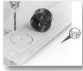
If the workpiece is especially thick ... ... it is also recommended that you cut from both sides, or drill a number of
