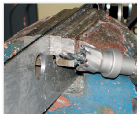
Free-hand drilling up to Ø 30 mm
