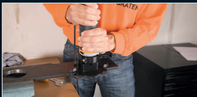
Initial drill-holes from: Ø 3.0 mm for pen cutters Ø 5.0 mm for spherical cutters
