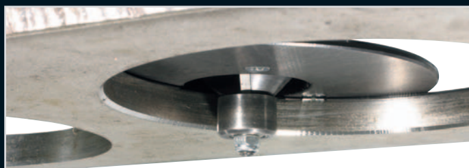
Start holes from Ø 20 mm.
