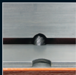
Position I: Material thickness from 4.5 mm
