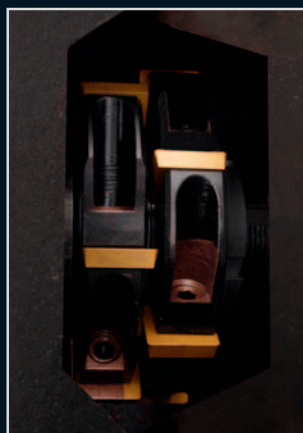
2 milling disks together with 6 inserts each
