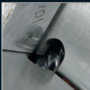
Exact deburring with with self-generating milling cutter
