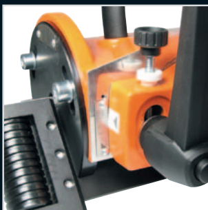
Fine adjustments to milling depth/bevel width
