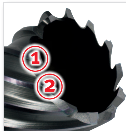
High-performance tothing with pre- (1) and post-cutting (2)
